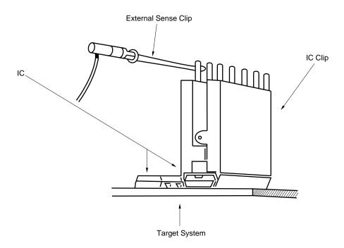
Figure 2-5. Connecting the External Sense Clip
