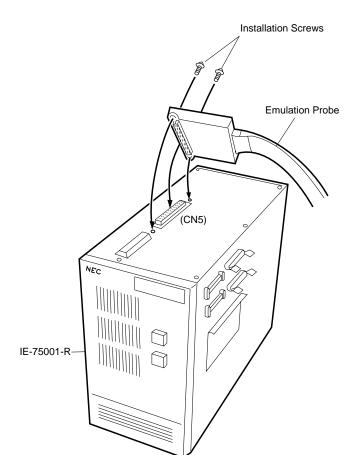
Figure 2-2. Connecting the IE-75001-R and Emulation Probe
