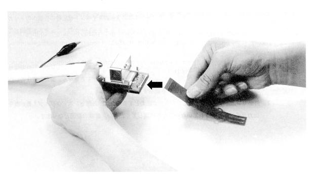
Figure 2-4. Emulation Probe Connection
